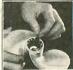
Shear-off Pin Compartment —Ingenious magazine in propeller hub houses extra pins. As handy as leads in an automatic pencil. Instantly withdrawn. Always ready—never lost or left ashore.
