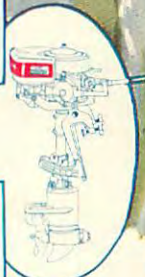
Johnson Big Twin Weight 85 lbs. 6 h. p. Speed 12 to 16 m. p. h.
